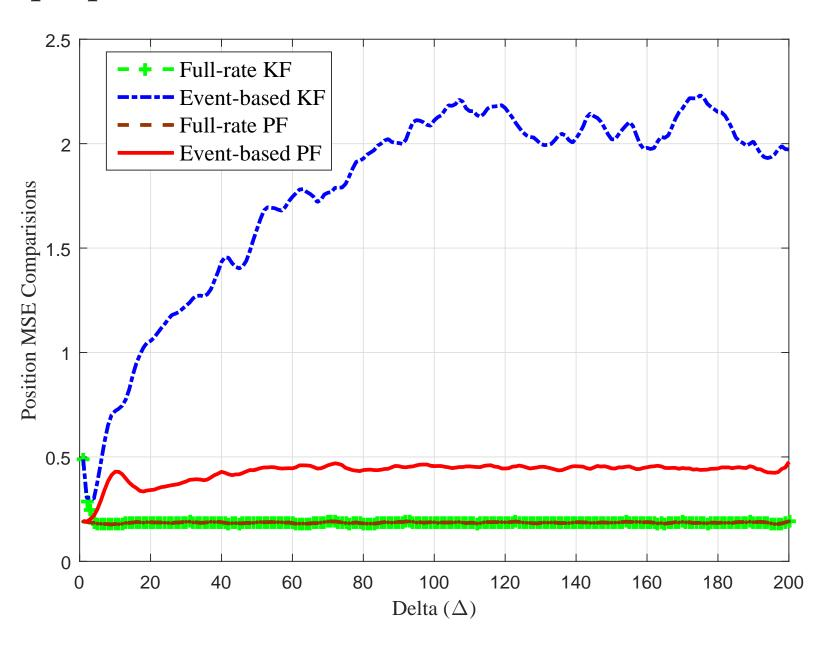
**Figure 1:** The Position MSE comparison when  $\Delta = 1.2$ .
