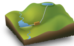
Pumped-storage Hydroelectric Power Plant
