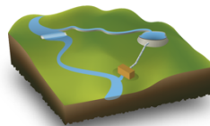
Derivational Hydroelectric Power Plant
