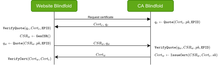
Figure 2: Interactions between a website and CA for certificate issuance during operational phase
