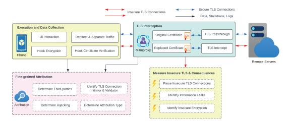
Figure 2: Components and workflow of Marvin
