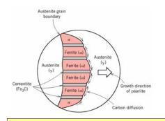
The layers of alternating phases in pearlite are formed for the same reason as layered structure of eutectic phases: redistribution C atoms between ferrite (0.022 wt%) and cementite (6.7 wt%) by atomic diffusion.
