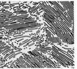
the dark areas are  $Fe_3C$  layers, the light phase is  $\alpha$  -ferrite
