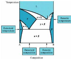
The above phase diagram contains both an eutectic reaction and (its solid-state analog) an eutectoid reaction
