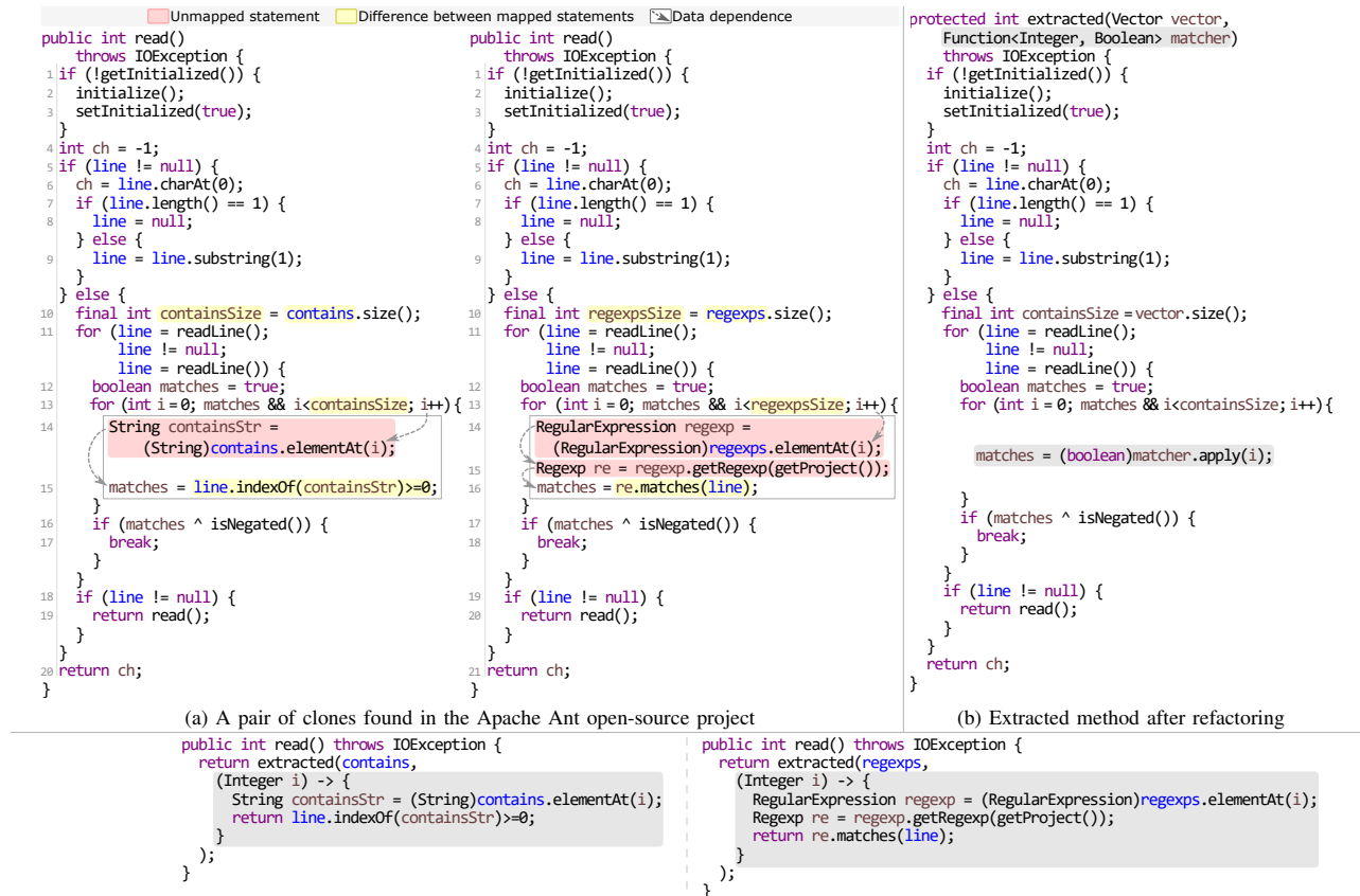
Fig. 2. Using Lambda expressions to enable the refactoring of Type-3 clones.
