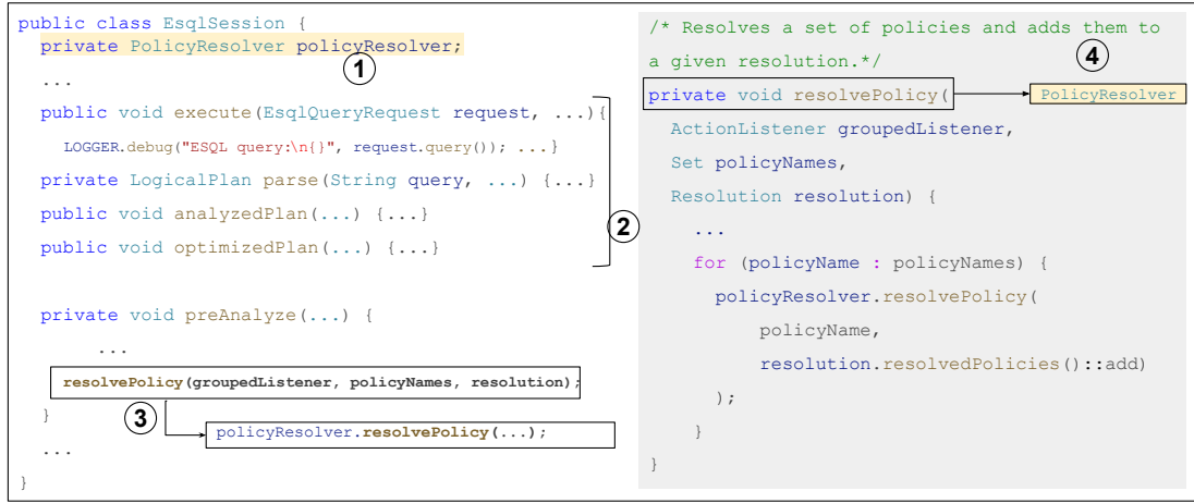
Fig. 1: A real-world example demonstrating a MOVEMETHOD on resolvePolicy performed by developers in the Elasticsearch project, commit 876e7015
