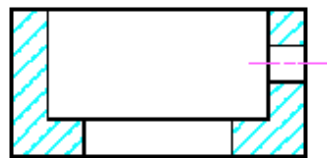
Incorrect cutting plane line
