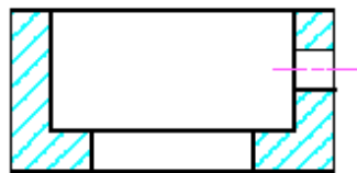
Correct cutting plane line
