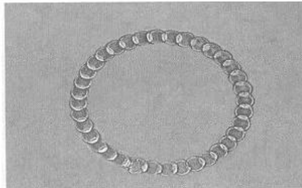
FIGURE 35-9 Seam welds made with overlapping spots of varied spacing.
