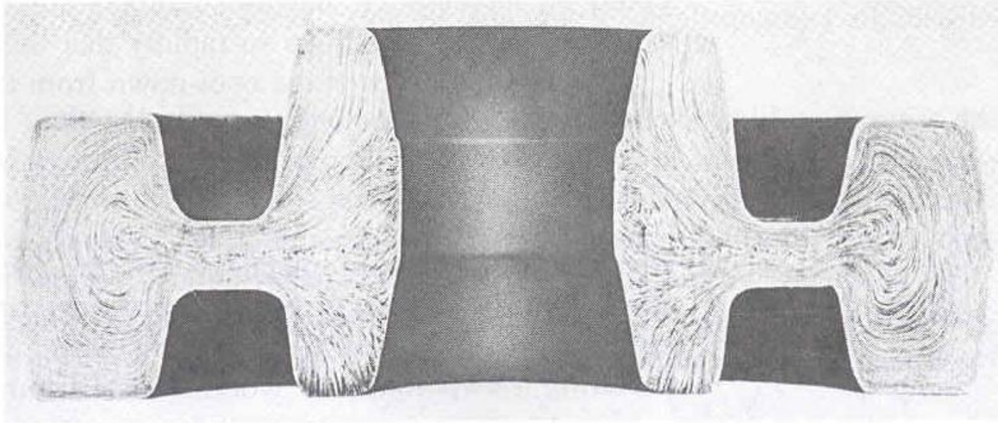
FIGURE 17-4 "Fiber" structure of a hot-formed (forged) transmission gear blank. (Courtesy of Bethlehem Steel Corporation.)
