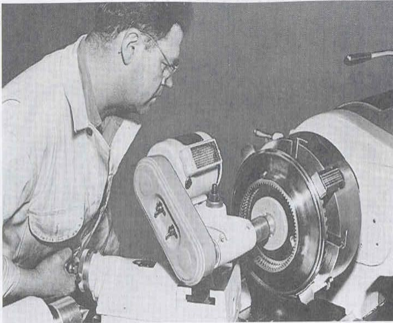
FIGURE 27-20 Grinding a bearing seat by means of a tool-post grinder on a lathe. (Courtesy of Dunore Company.)
