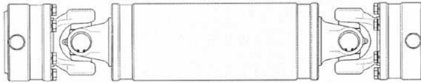
Figure 3.1: Cardan Joint, used in Trucks
