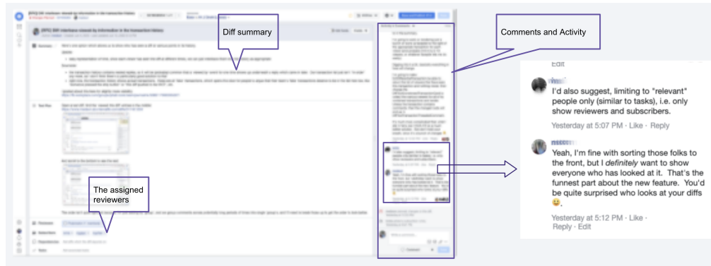
Figure 1: A redacted view of a diff under review in DiffTool. Authors and reviewers can interact via the diff review page in Phabricator. The diff under review has several sections including the diff summary, the actual changes that happened, the assigned code reviewers, the interactions between the various reviewers and author, the test case information and status, the results of static analysis, historical information etc.
