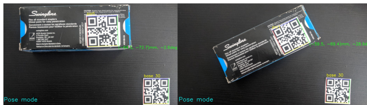
Figure 8. Use of two QR codes for locating parts of different positions and orientations.
