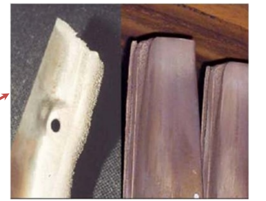
LDE damage to LP steam turbine blades
