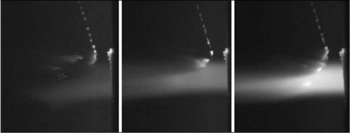
Figure 1-2 Radial injection of the liquid carrier into the plasma jet showing the jet fluctuations effect on the feed penetration into the plasma core [43]
