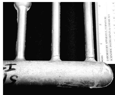
Fig. 5. Tears in a casting produced with an alloy having low resistance to hot-tearing.
