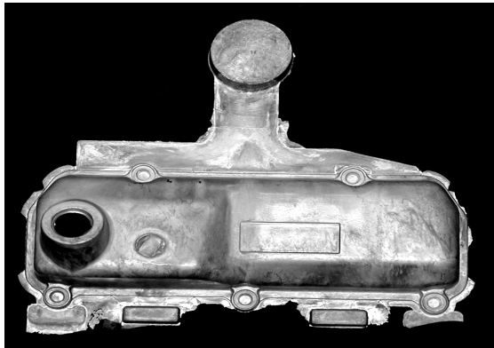
Fig. 6.a. Valve-cover cast in AJ52x at Spartan Light Metal Products with very good results.
