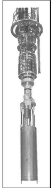
Fig. 6.8. Miscibility gap in He 3 -He 4 phase diagram (schematic). Enriching He 3 in the He 3 -rich phase by evaporation. He 3 -He 4 cryostat of the Physikalisch Technische Bundesanstalt in Berlin. 33
