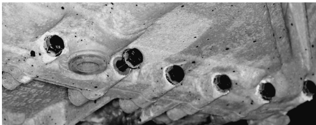
Figure 10b: Mg gearbox housing after 12 cycles of dynamic corrosion testing (EK3); with the bolted joint "zinc plus olive-chromated plus KTL"
