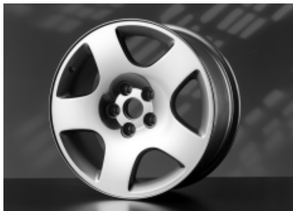
Figure 14: Prototype of a magnesium forged wheel (ZK30), produced on the basis of the corresponding aluminium part, which is already in series production for the Audi A8 (wheel size: 8Jx17)
