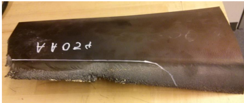
Figure 3.12 Eroded blade with sever erosion marks
