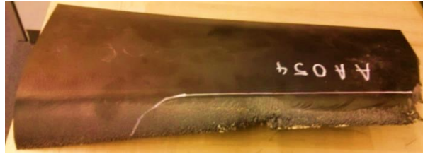
Figure 1.2 Eroded ex-service turbine blade
