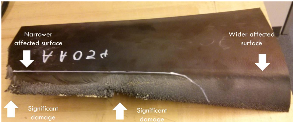
Figure 6.2 Eroded surface area of Blade 2
