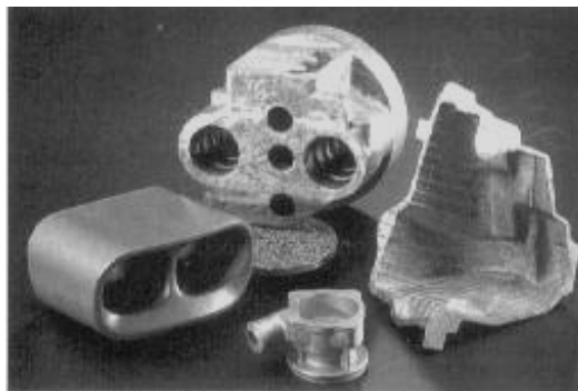
Figure 1.16: Applications of metallic foams in manufacturing automobile parts such as gear box case or pipe connectors [33].
