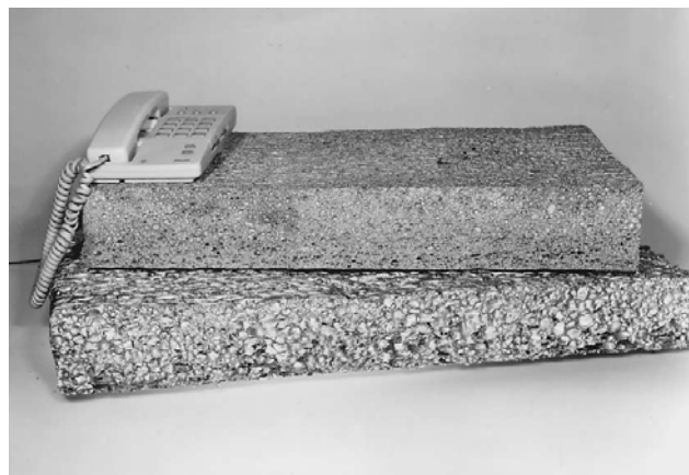
Figure 1.7: Foam slabs of two different densities and cell sizes produced by the gas injection method (sample: Hydro Aluminum, Norway) [12].
