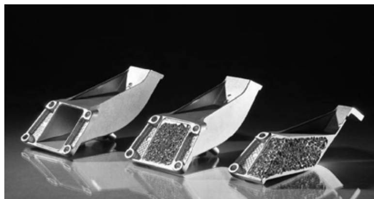
Figure 1.19: Prototype of a BMW engine mounting bracket manufactured by LKR Ranshofen (Austria). From left to right: empty casting, entire composite part consisting of foam core and cast shell, section through composite part (courtesy of LKR).
