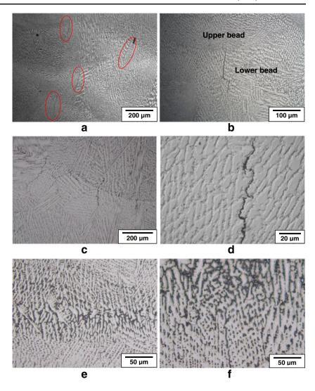
finest structure resolvable using optical microscopy and represents the low angle boundaries separating the various morphological forms of solidification, such as cells, dendrites, and cellular dendrites. The SGBs are formed at the intersections of packets of SSGBs with different grain growth directions and therefore represent high-angle grain boundaries. In contrast, the MGBs were frequently observed in the CZ in
