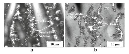
IN718 welds and castings [4–6, 27, 28]. Therefore, the Laves phase is detrimental and hence should be carefully controlled. Compared with the ADed condition (Fig. 7a and b), less Laves particles are observed in the interdendritic regions after the PCHT (Fig. 7c and d). Thus, the PCHT results in considerable dissolution of the Laves particles at a solution temperature of 954 °C. In this case, less interdendritic constituents
