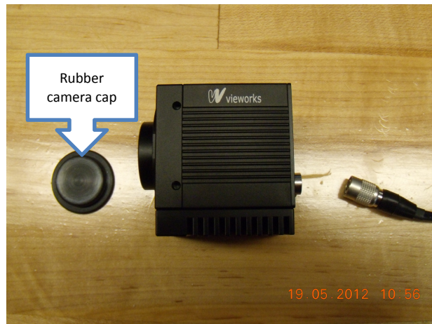
Figure 31: Once Lens removed cap camera to protect CCD chip.
