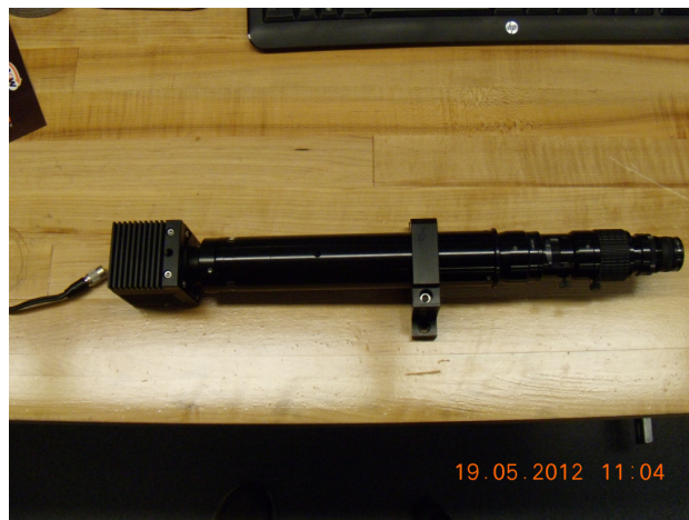
Figure 30: Vieworks camera must be unplugged prior to removing lens and capping.
