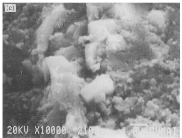
Fig. 10. Fracture surfaces in bending (SEM) of the SHS-processed in situ composites (a) \text{TiB}_2/\text{Al} , (b) and (c) \text{TiC}/\text{Al} .
