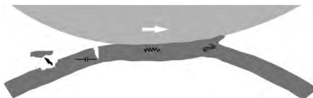
Fig. 3.94. Micromechanical tribological mechanisms consider stress, strain, crack generation and propagation and single particle formation on a microlevel, typically this is what takes place in asperity contacts.
