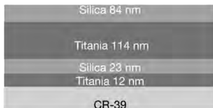
Fig. 7.26. A typical four-layer \text{SiO}_2/\text{TiO}_2 anti-reflection coating design on plastic (thermoset cast CR-39) eyeglass lenses (after Colton, 1997).
