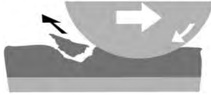
Fig. 3.99. Fatigue wear is characterized by repeated loading of the coated surface resulting in cracking at the surface in the coating, followed by fracture, material detachment and debris generation.
