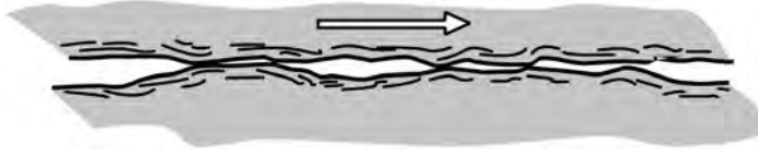
Fig. 3.14. Parallel subsurface cracks and plate-like wear debris are formed as a result of repeated loading in delamination wear.
