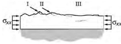
Fig. 4.53. Model for the wear process of brittle diamond coatings subjected to high compressive biaxial stresses resulting in surface smoothing (after Gunnars and Alahelisten, 1996).
