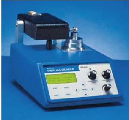
Figure 6.12. A dimpling grinder for thinning metallic specimens to a few micrometers thick prior to ion beam milling (Picture courtesy of Fischione Instruments, Pittsburgh, PA)
