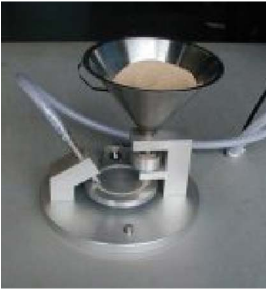
Figure 6.11. The fine sand feed on a gas jet erosion system. The high pressure gas jet is to the left of the picture (Picture courtesy of Phoenix Tribology Ltd., USA)
