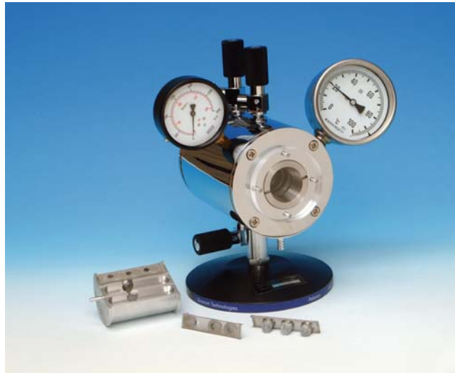
Figure 7.8. The Quorum Technologies E3100 large chamber critical point dryer with specimen containers and the boat to transfer the specimens into the critical point drier (Picture courtesy of Quorum Technologies, Ringmer, Sussex, UK)
