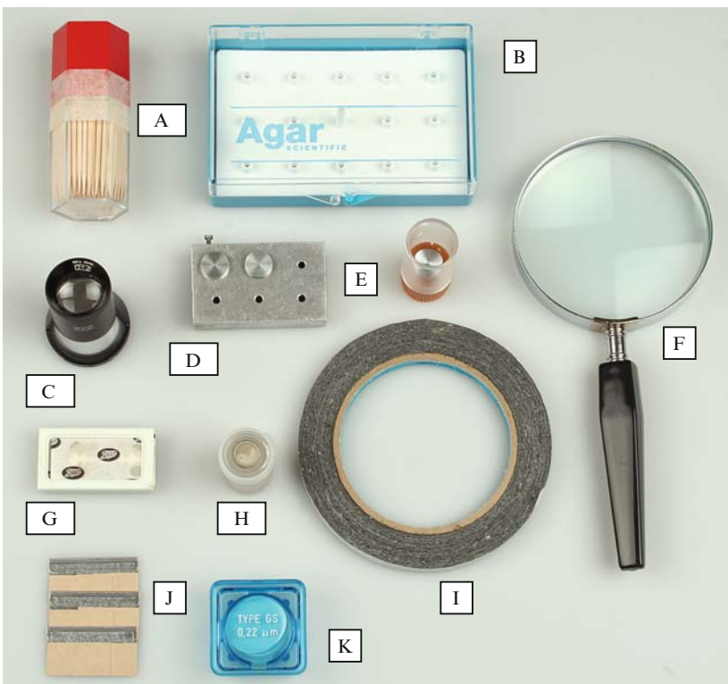
Figure 3.10. A. Wooded tooth picks. B. Large plastic specimen storage box. C. small \times 10 hand lens. D. Working aluminum holder for 12-mm stubs. E. Secure container for a single stub. F. Large \times 4 hand lens. G. Very thin razor blades. H. Container of Silver-Dag suspension. I. Double-sided conductive adhesive tape. J. Thick razor blades. K. Fine-pore Millipore filters
