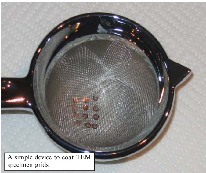
Figure 4.3. Twelve 3.05-mm 400 mesh copper grids covered with a thin Formvar film and trapped at the base of a 50-mm diameter stainless steel tea strainer
