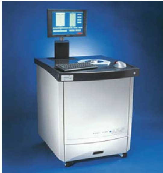
Figure 6.19. An automatic sample preparation system that will plasma clean, ion beam etch, reactive ion beam etch, reactive ion etch, and carry out high resolution ion beam sputter coating (Picture courtesy of Fischione Instruments, Pittsburgh, PA)
