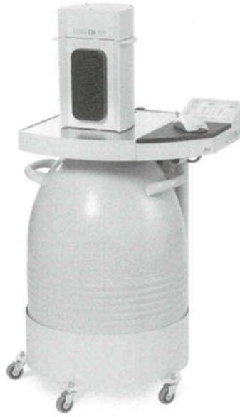
Figure 7.15. Leica EM AFS2 portable freeze substitution device situated on a large liquid nitrogen Dewar (Picture courtesy of Leica Microsystems GmbH, Vienna, Austria)
