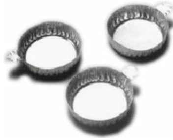
Figure 5.3. Disposable aluminum trays for embedding large samples. Picture courtesy of Agar Scientific (Stansted, UK)
