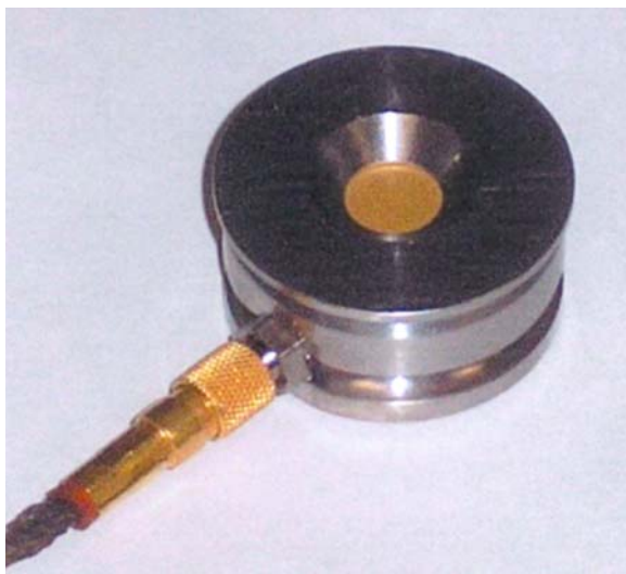
Figure 11.22. The type of quartz thin film monitor used to measure thin film thickness during coating of SEM specimens. The monitor is at the centre with an area of 5\text{mm}^2 and the connections lead to an exterior monitor
