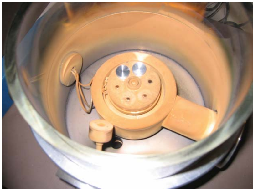
Figure 11.12. A view of the inside of a badly contaminated sputter coater. There has been no attempt to either clean the bell jar or the surface on which the specimen holders are placed
