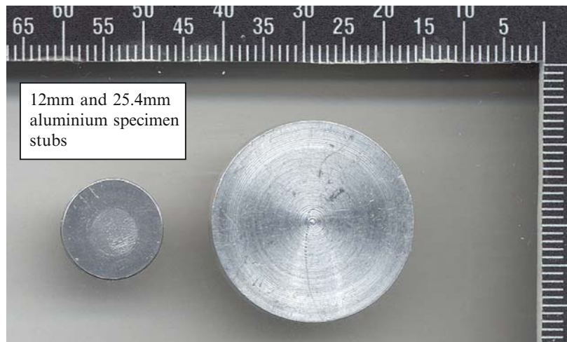
Figure 3.1. 12- and 24.5-mm aluminum specimen stubs
