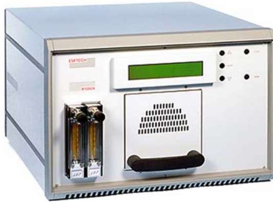
Figure 6.13. Plasma etcher used for cleaning and removing organic material from sample to be examined in the SEM (Picture courtesy of Quorum Technologies, Ringmer, UK)
