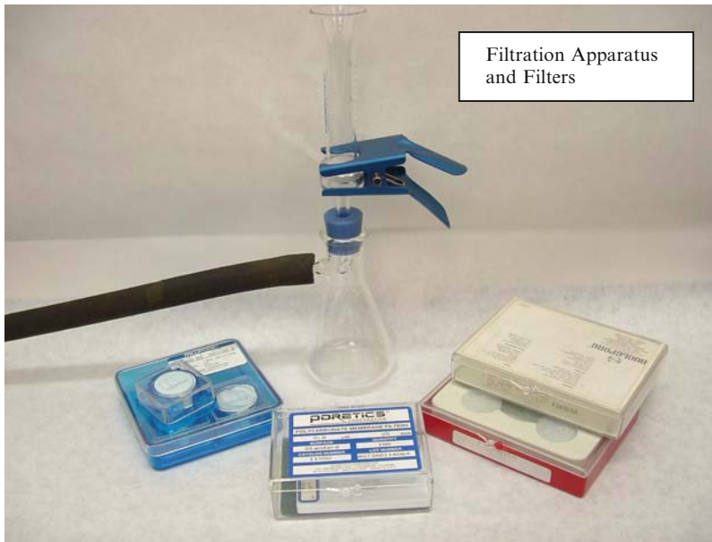
Figure 3.3. Filtration apparatus and filters composed of a system that allows a liquid suspension to pass through filters of various size designed to retain solids of different sizes and compositions
