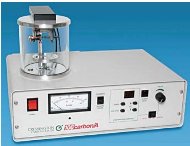
Figure 11.9. An Auto Carbon Coater for producing thin films on non-conductive SEM specimens for x-ray microanalysis. Picture courtesy Ted Pella Inc, Redding, California, USA
