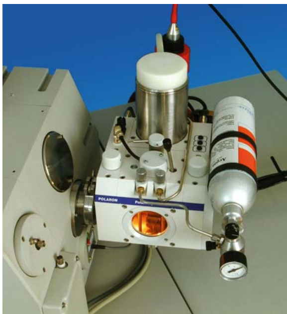
Figure 8.17. The Quorum technologies PP2000 integrated low temperature preparation and SEM cold stage (Picture courtesy of Quorum Technologies, Ringmer, Sussex, UK)
