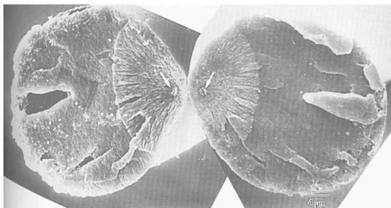
Figure 6.2. A pair of complementary fractures of a polyethylene terephthalate (PET) fiber. The arrows show a defect at the locus of the failure (Picture courtesy of Sawyer et al., 2008)
