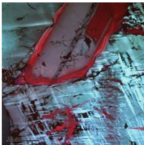
Figure 9.6. An SEM cathodoluminescence image of a polished piece of granite from Llano, Texas. The bluish cross hatched area is potassium feldspar and the purple-red area is sodium feldspar. Picture courtesy Juergen Schieber, Department of Geology, Indiana University, USA
