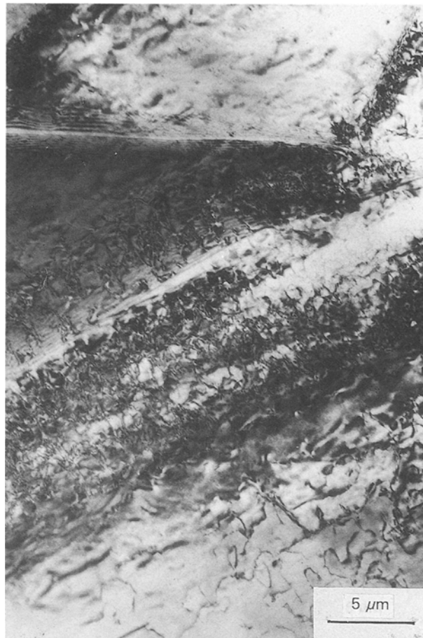
Figure 5 A high dislocation density and heavy twinning around the SiC particles.
