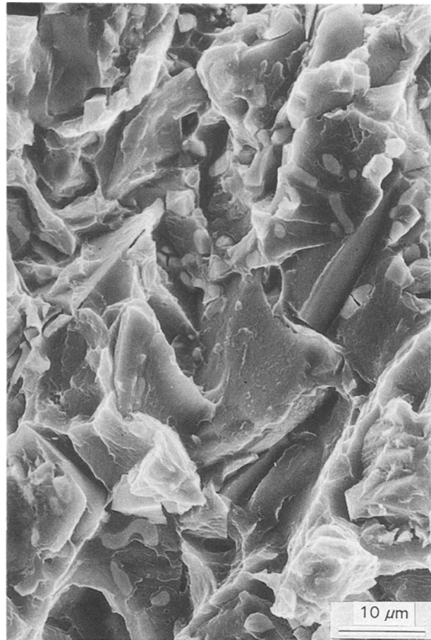
Figure 7 A thin magnesium layer on the SiC particle surface.
