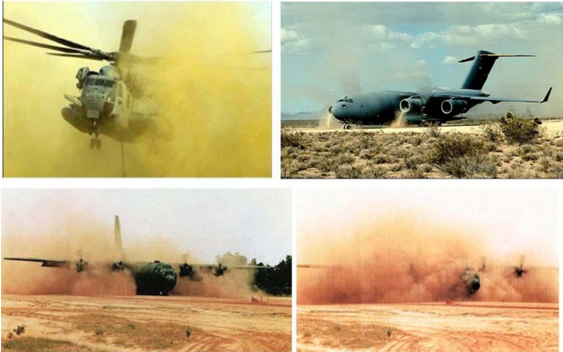
Figure 1-2 Examples of severe solid particle erosion environments in flight engines. Nano-scale PVD coatings have been used to improve turbine durability and reliability.
