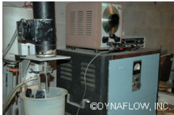
b) ASTM G-32 Cavitation Erosion Test System
