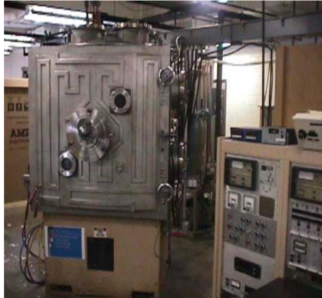
Figure 2-12 Praxair CA-PVD coater # 3 with multiple arc cathodes, a load capacity of 400 lbs (181 kg) (rotation mode), and a coating zone 30 inches (76 cm) in diameter and 36 inches (91 cm) in height
