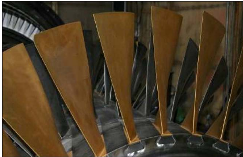
Figure 2-30 T-Armor coated Frame7 FA R0 compressor blade row
