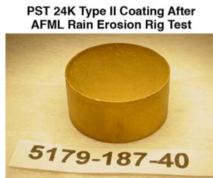
Figure 2-19 Praxair 24K+ Type 2 TiN coating rain erosion test sample after 450 minutes [70]
