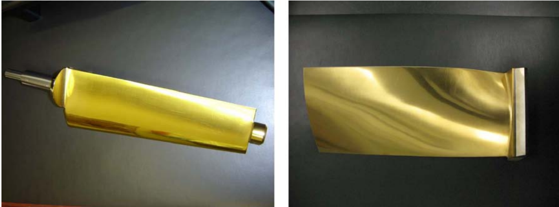
Figure 2-8 Frame 7EA VGV compressor inlet vane and Fr 7FA Row 0 compressor blade coated with Liburdi RIC erosion-resistant coating [53]
