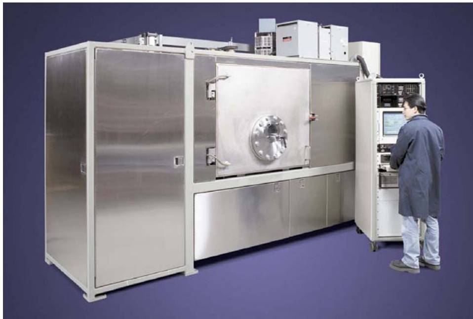
Figure 2-3 Liburdi RIC large production coating unit. Effective coating zone 1.2 x 1.2 x 1 m (3.9 x 3.9 x 3.3 ft). Capable of coating multiple larger IGT compressor blades.
