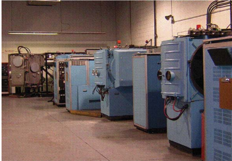
Toronto Coating Facility Four Deposition Systems SP-1000 (1.0 m 3 - 35 ft 3 Capacity) and Prototype SP-2000 (2.0 m 3 - 70 ft 3 Capacity)
