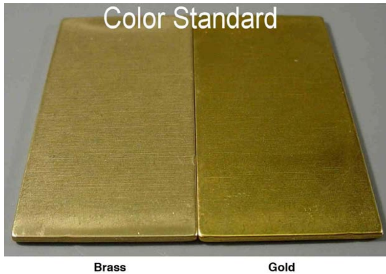
Figure 2-14 Praxair 24K color comparison between sub-stoichiometric (left) and fully stoichiometric TiN (right). The coating color is used as a quality control metric.
