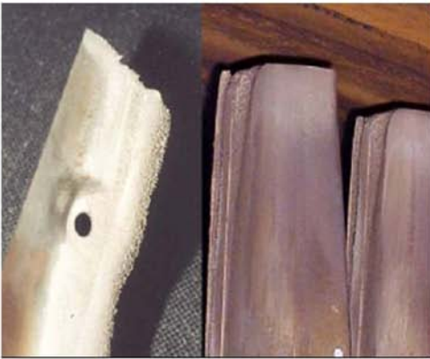
c) LDE Damage to LP Steam Turbine Blades
