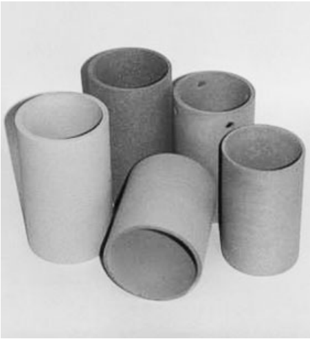
Fig. 3.18 Preforms to reinforce cylinder running surfaces.
