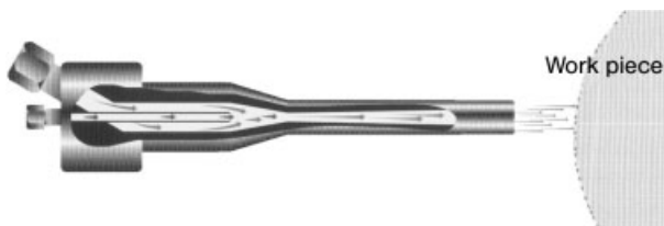
Fig. 5.10 Principle of cold gas spraying (Linde AG).
