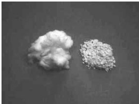
Fig. 3.7 Fiber wool: left, bulk fiber; right, milled fiber
