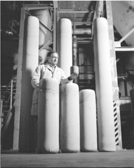
Fig. 11.12 Spray formed billets of PEAK Werkstoff GmbH.
