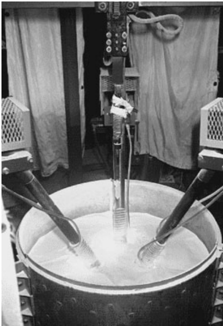
Fig. 3.2 Fiber melting furnace, top view.
