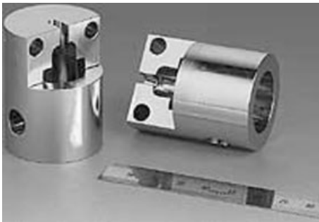
Fig. 10.26 Clamping device for test engineering at high temperatures of PM 2000 [2, 51].
