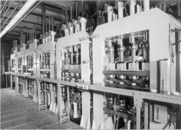
Fig. 3.11 Preform series production equipment, press side.
