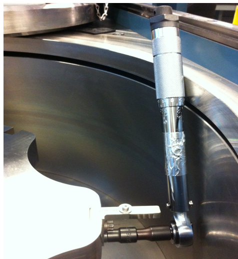
Figure 4: Torqueing the sample bolts
