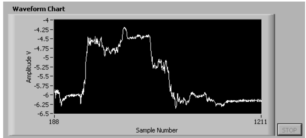
Figure 7.10 Waveform Chart used to display acquired data point by point.
