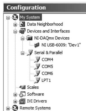
Figure 5.22 Expanding the Devices and Interfaces node.
