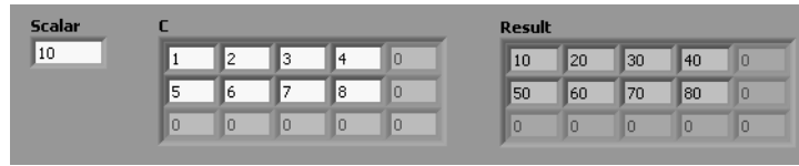
Figure 4.18 Multiplying an array by a scalar (front panel).
