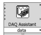
Figure 5.33 The DAQ Assistant Express VI on the block diagram after configuring the task.
