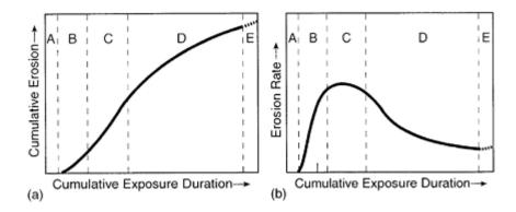
For bulk materials determination of incubation period and maximum erosion rate are the objected. After which empirical relationships can be used to determine these parameters at differing liquid impingement conditions.
