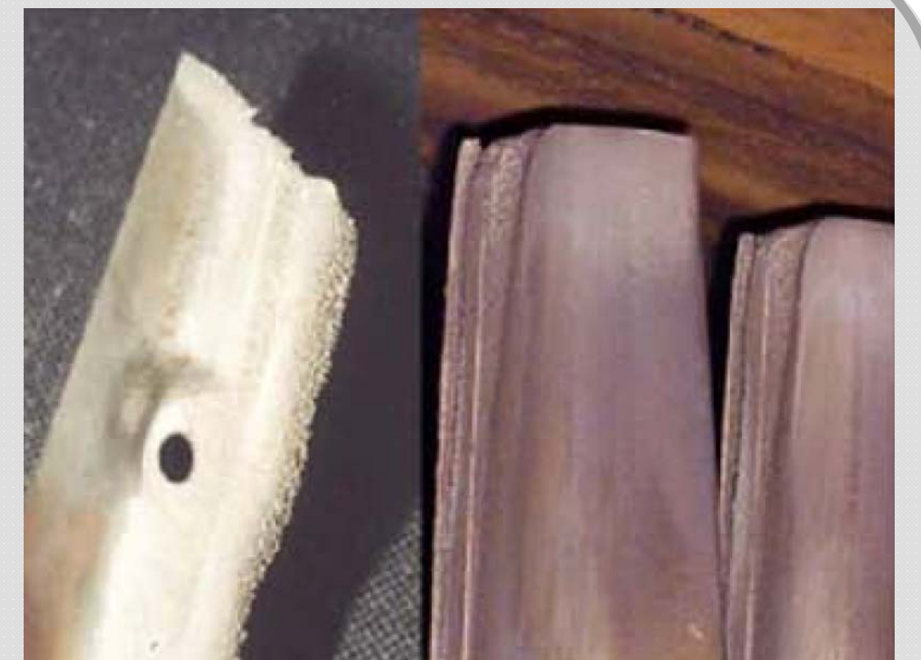
Real Blades Damage via Water Droplet Erosion [Reference: EPRI Report 2008]
