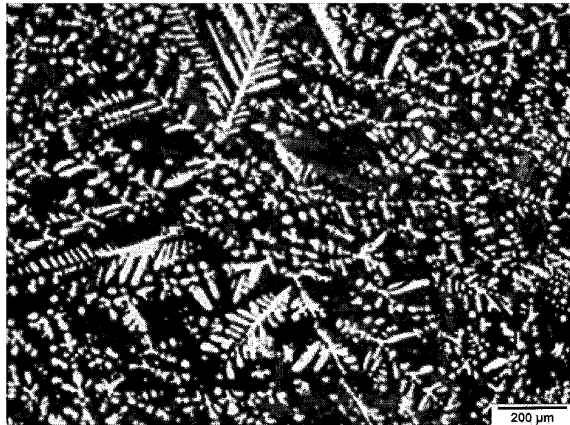
Figure 5-54: (Mg) dendrite of sample 11 100X (12.65/77.46/9.89 Ca/Mg/Al wt%.)
