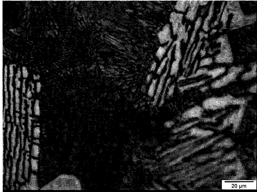
Figure 5-60: Optical microscope of sample 12, 1000X (19.32/62.65/18.04 Ca/Mg/Al wt%)
