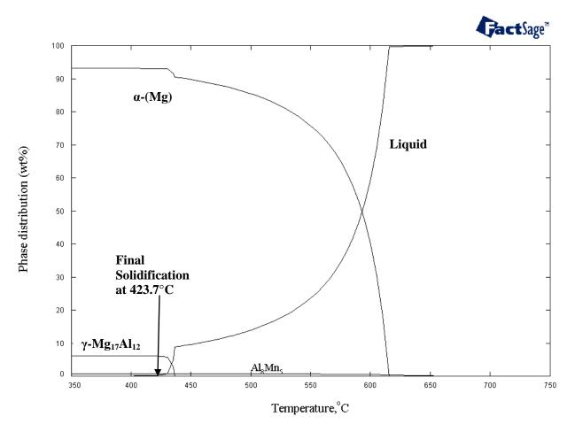
Figure 39: Scheil phase distribution of AM60B alloy
