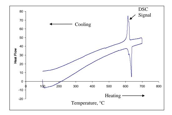
Figure 25: A DSC spectra of the AE44 alloy at 5°C/min scanning rate
