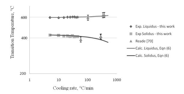
Figure 53: Extrapolation of the transition temperatures of AZ91D to high cooling rates in double logarithmic graph
