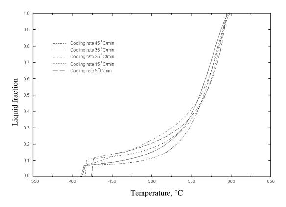
Figure 20: Solidification curves of AZ91D at different cooling rates drawn from the experimental data using HTM
