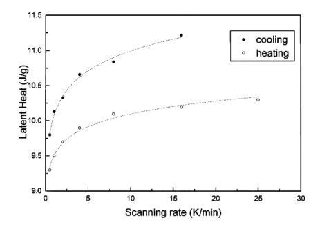
Figure 8: The effect of scanning rates on the latent heat of pure Co [37]
