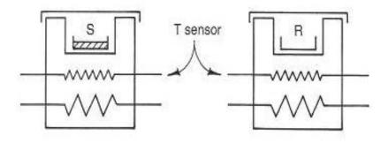
Figure 12: The principle of power compensated Differential Scanning Calorimeter Analysis [48]
