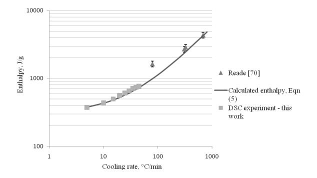
Figure 50: Extrapolation of latent heat of solidification of AZ91D to high cooling rates in double logarithmic graph
