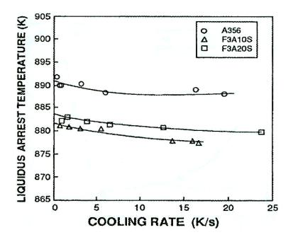
Figure 5: Liquidus temperature vs. cooling rate for three different Al-Si alloys [31]
