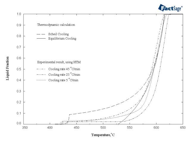
Figure 32: Comparison between experimental and calculated solidification curves of AM60B alloy
