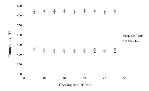
Figure 23: Transformation temperatures of AM60B alloy at different cooling rates
