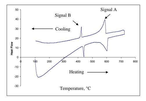
Figure 17: DSC spectra of AZ91D at 5°C/min scanning rate
