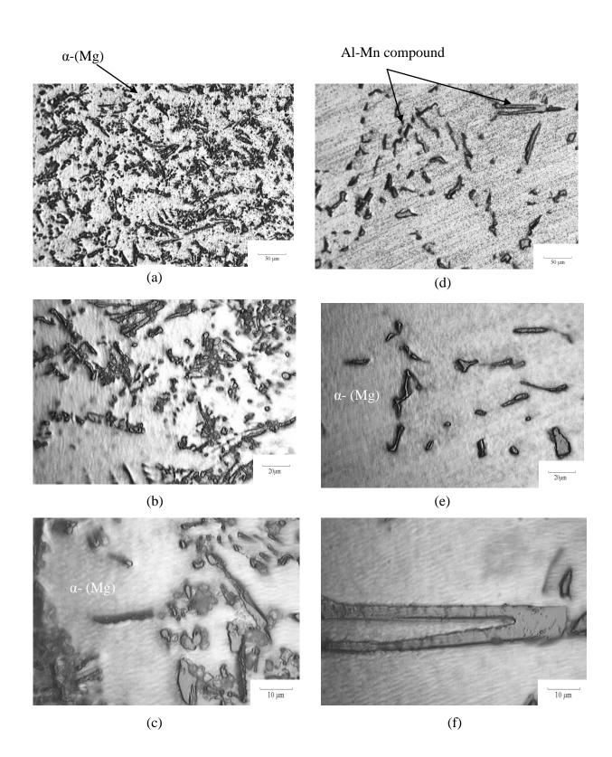
Figure 47: As-cast microstructure of AE44 ( a) 100X (b) 500X (c) 1000X; Post-DSC microstructure of AE44, DSC cooling rate 5°C/min (d) 100X (e) 500X (f) 500X
