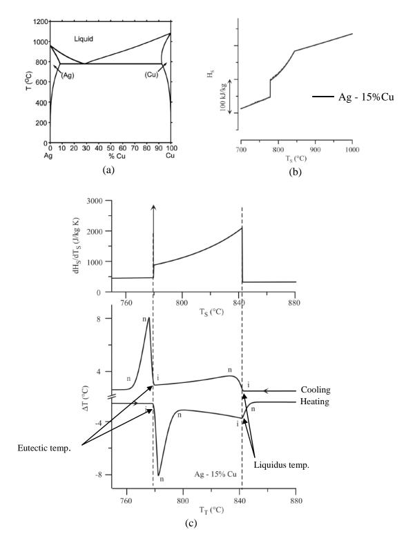
Figure 11: (a) Ag-Cu phase diagram, (b) enthalpy vs. temperature curve for Ag-15% Cu alloy (c)  $dH_{s}/dT_{s}$  vs.  $T_{s}$  curve and computed DTA scan for Ag-15% Cu alloy [52]
