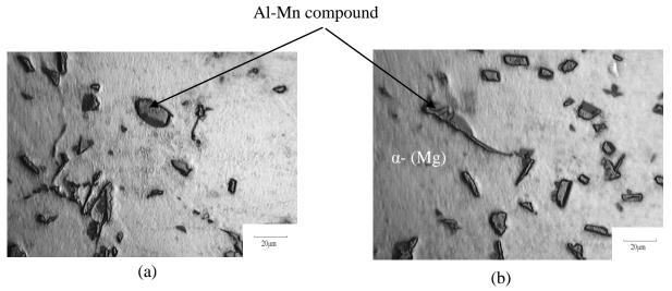
Figure 49: Post-DSC microstructure of AE44, DSC cooling rate  $20^{\circ}$ C/min, (a) 500X (b) 1000X
