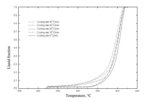
Figure 24: Solidification curve of AM60B alloy drawn from the experimental data using HTM
