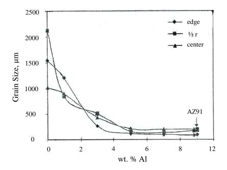
Figure 4: Effect of Al content on grain size of pure Mg [22]
