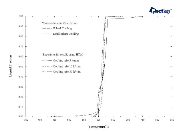
Figure 34: Comparison between experimental and calculated solidification curves of AE44 alloy
