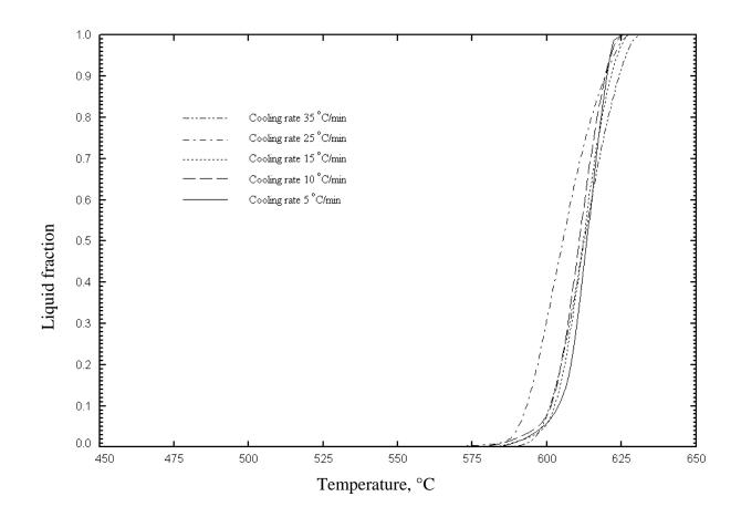
Figure 28: Solidification curve of AE44 drawn from the experimental data using HTM
