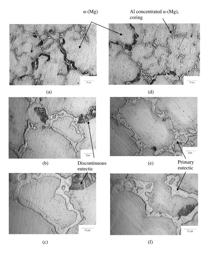
Figure 43: Post-DSC microstructure of AZ91D, DSC cooling rate 25°C/min: (a)100X (b) 500X (c) 1000X; Post-DSC microstructure of AZ91D, DSC cooling rate 45°C/min: (d) 100X (e) 500X (f) 1000X
