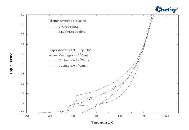
Figure 30: Comparison between experimental and calculated solidification curves of AZ91D
