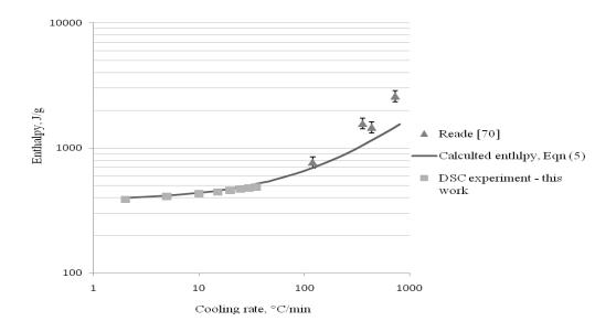
Figure 52: Extrapolation of latent heat of solidification of AE44 to high cooling rates in double logarithmic graph
