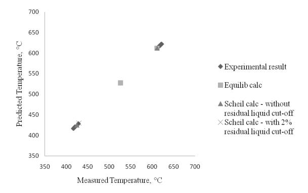
Figure 33: Comparison between experimental and calculated transition temperatures of AM60B alloy of AM60B alloy
