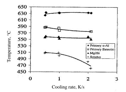
Figure 7: Plot of phase transformation temperatures of primary α-Al, Primary eutectic, Mg<sub>2</sub>Si and solidus temperature in AA5182 aluminum alloy at different cooling rates [33]
