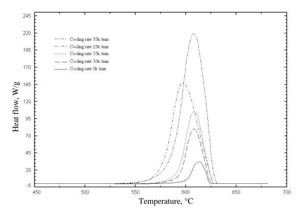
Figure 26: DSC spectra of AE44 alloy at different cooling rates after subtracting the baseline
