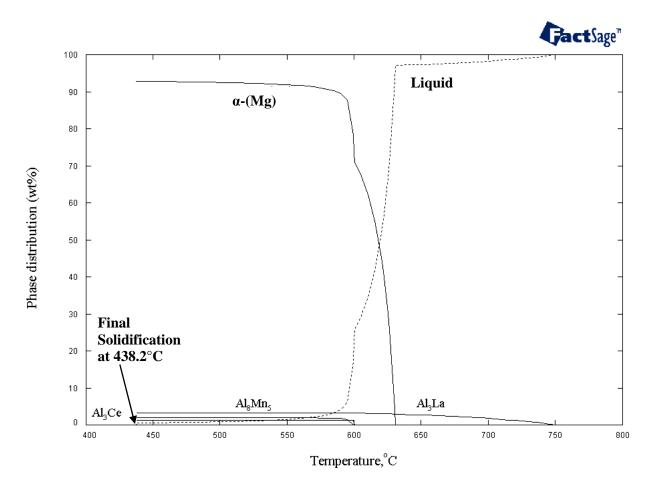
Figure 41: Scheil phase distribution of AE44 alloy
