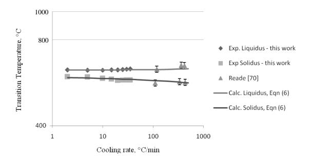
Figure 55: Extrapolation of the transition temperatures of AE44 to high cooling rates in double logarithmic graph
