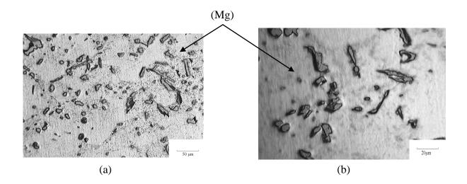
Figure 48: Post-DSC microstructure of AE44, DSC cooling rate  $10^{\circ}$ C/min, (a) 500X (b) 1000X
