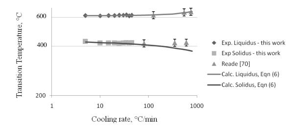
Figure 54: Extrapolation of the transition temperatures of AM60B to high cooling rates in double logarithmic graph
