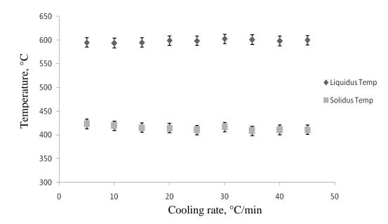
Figure 19: Transformation temperature of AZ91D at different cooling rates
