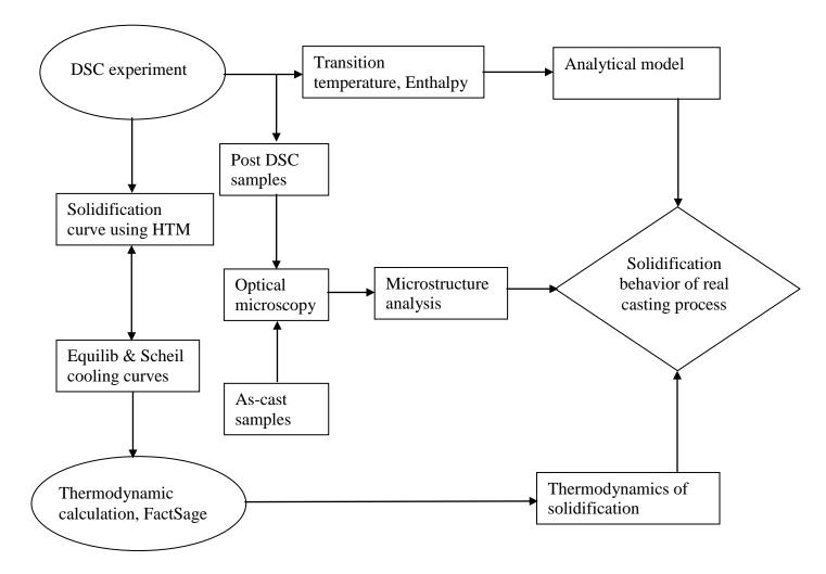
Figure 16: Flow chart illustrating the methodology of the current work
