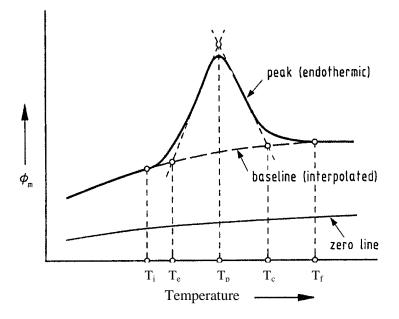
Figure 14: Definition of zero line, baseline, and characteristic temperatures [51]
