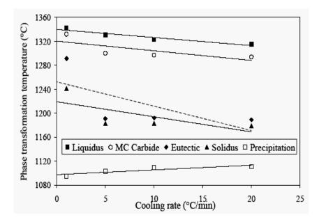
Figure 6: Phase transformation temperatures of Inconel 738LC nickel based super alloy at different cooling rates [35]
