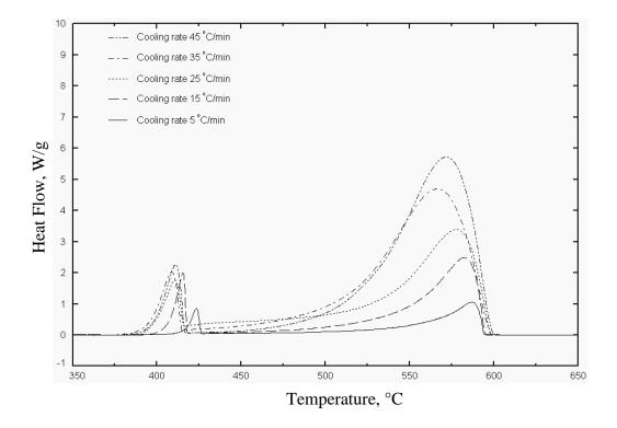
Figure 18: DSC spectra of AZ91D alloy at different cooling rates (after subtracting the baseline)
