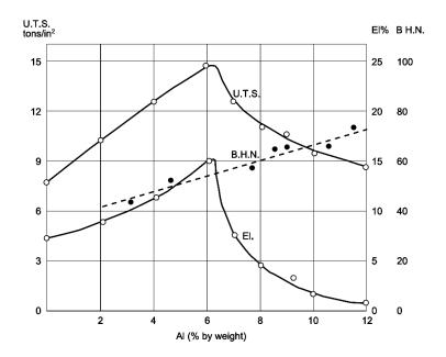
Figure 3: Effect of Al content on ductility (sand cast sample, as cast condition) [21];
