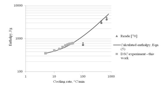
Figure 51: Extrapolation of latent heat of solidification of AM60B to high cooling rates in double logarithmic graph
