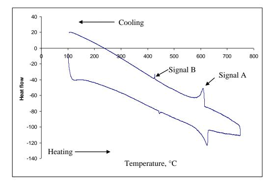
Figure 21: DSC spectra for AM60B at 5°C/min scanning rate
