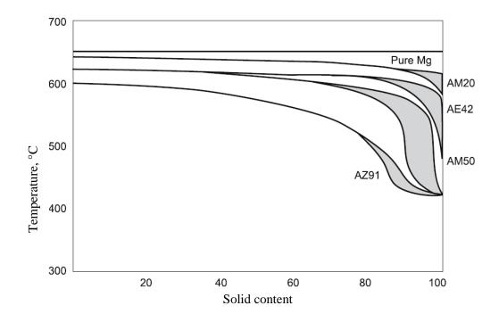
Figure 9: Solid content as a function of temperature for Mg-Al alloys [39]
