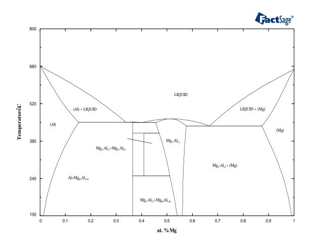
Figure 2: Mg-Al binary phase diagram [19]
