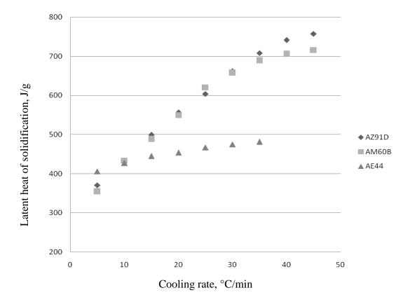
Figure 29: Change of latent heat of solidification of the alloys at different cooling rates
