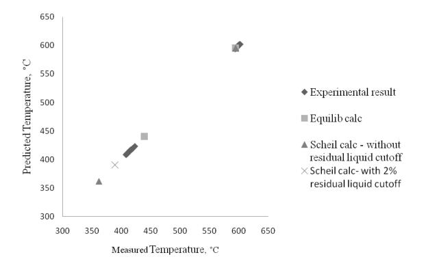
Figure 31: Comparison between experimental and calculated transition temperatures of AZ91D alloy
