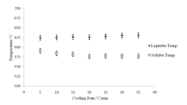
Figure 27: Transformation temperature of AE44 alloy at different cooling rates
