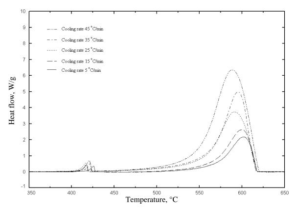
Figure 22: DSC spectra of AM60B alloy at different cooling rates after subtracting the baseline
