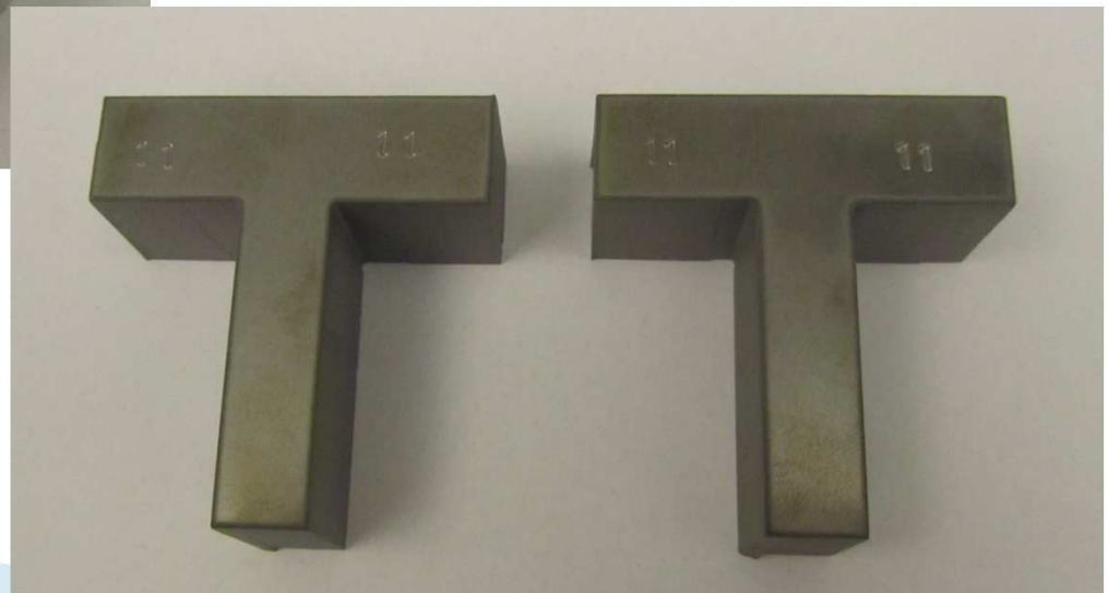
Disk #11 after water jet cutting
