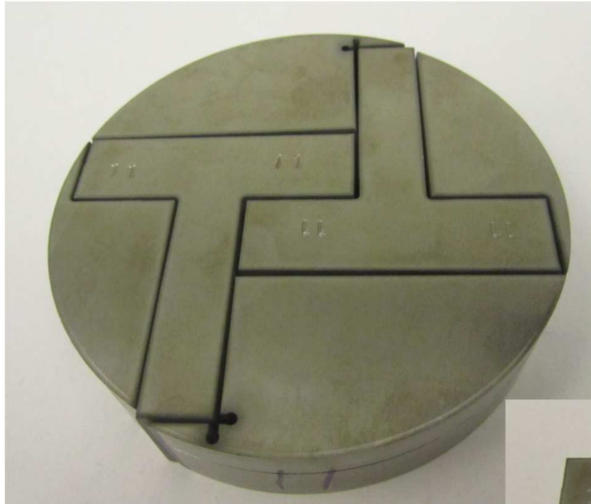
Disk #11 after water jet cutting
