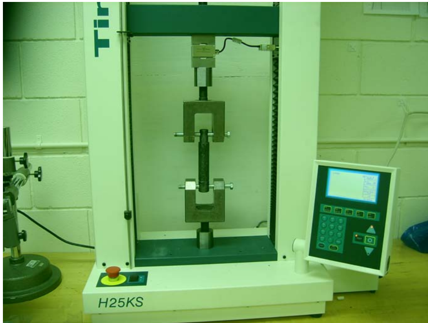
Figure 3-22: Tinius Olsen shear tester
