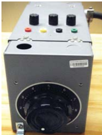
VARIAC , SHOWING FUSES [WITHOUT FUSE- STATUS INDICATOR BOX]
