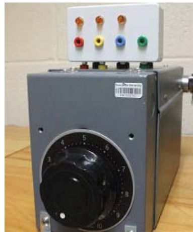
VARIAC, [WITH FUSE-STATUS INDICATOR BOX MOUNTED]
